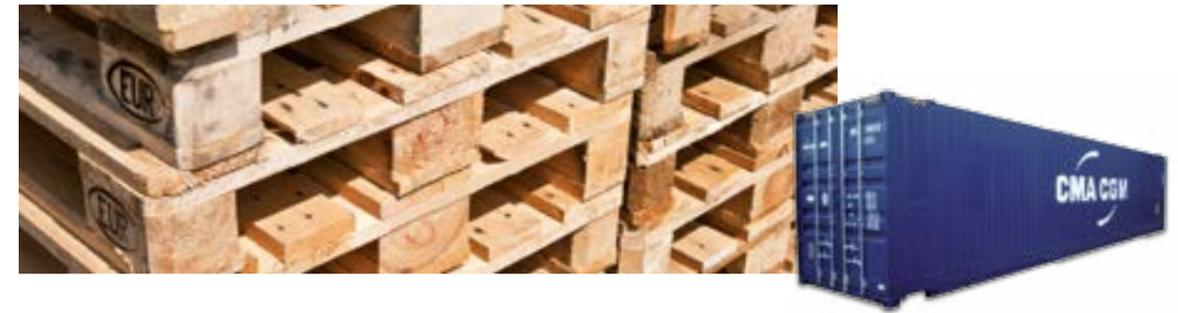
**Definition:** 40'/45' High Cube PalletWide units were specifically designed with the 1.2 m "Europallet" in mind. The equipment, with its internal width, allowing loading of 2 pallets side by side, ensures optimum utilisation of space. Shippers benefit by being able to load more Europallets than they would in a standard ISO container.
