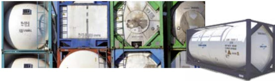
**Definition:** A freight container which includes two basic elements, the tank and the framework.
